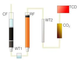
CF = Combustion Reactor WT1 = Water Trap (Physical) RF = Reduction Reactor WT2 = Water Trap (Chemical)
